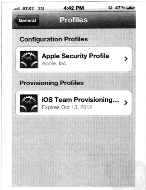
Figure 9-4. Forged configuration profiles do not alert the user to the fact that they are unsigned until clicked on.
