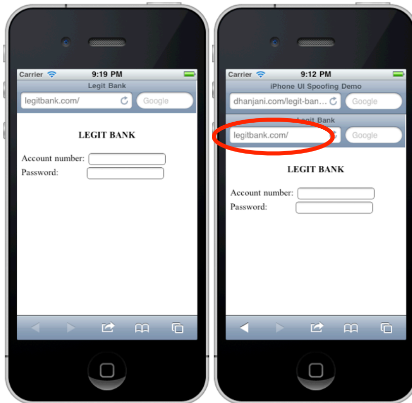
Figure 6: Image on the left illustrates the page rendered, which displays the 'fake' URL bar while the real URL bar is hidden above. Image on the right illustrates the real URL bar that is visible once the user scrolls up.
