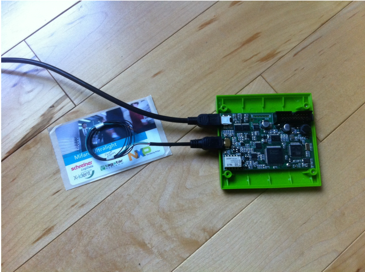
Figure 4: Proxmark homemade antenna waiting for a Type 2 transaction from a SCL3711
