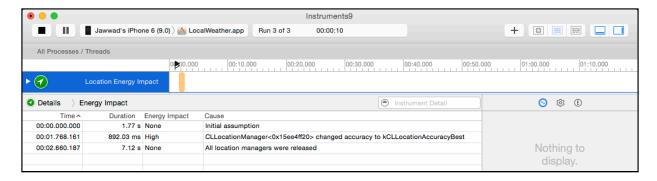
Notice the second row that says "CLLocationManager changed accuracy to kCLLocationAccuracyBest". The Energy Impact column shows High and the duration shows 892.03 ms.
