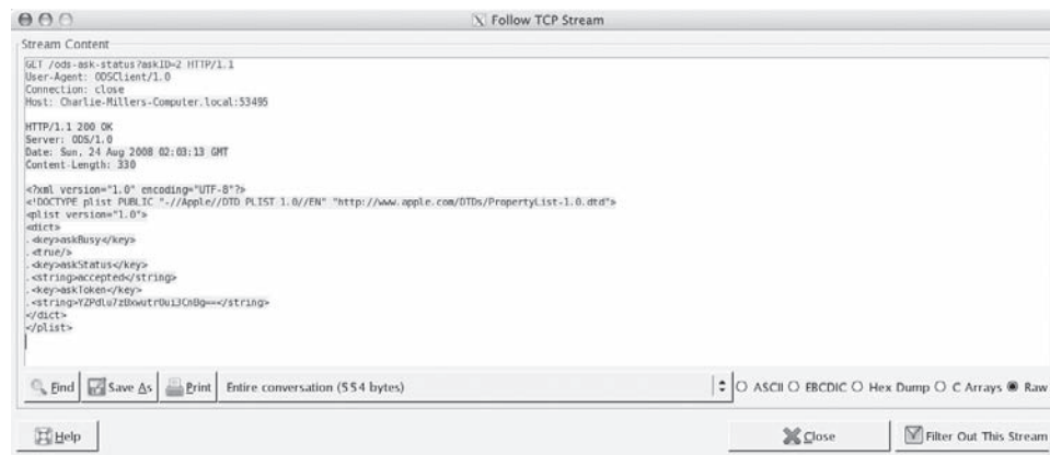
Figure 3-2: The data from a packet capture of a remote disk being authenticated
