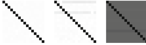
Fig. 3. Comparison of Cache Templates (address range of the first T-table) generated using Flush+Reload (left), Flush+Flush (middle), and Prime+Probe (right). In all cases k_0 = 0x00 .
