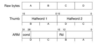
Fig. 3. Example decoding of four consecutive bytes of little endian instruction memory into two 16-bit Thumb halfwords and an ARM instruction with both a condition flag and an ALU destionation register. Bytes are denoted A-D. Note the correspondence between the first 4 bits of each Thumb halfword and the condition code and Rd.
